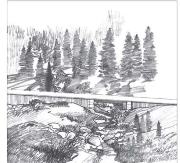
B | Intermittent and perennial streams should be bridged to preserve their hydrologic function and visual quality.
