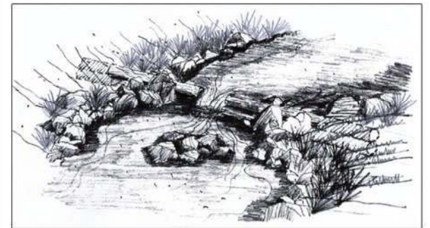
C | Drop structure using indigenous log construction.
