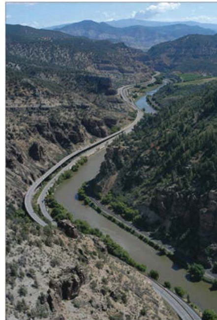
D | The roadway should respect the sinuosity of the valley floor and creek.
