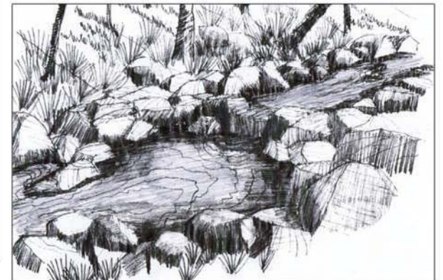
D | Drop structure using indigenous rock construction.
